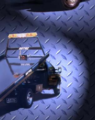
Specially designed for the Ford F-Series, the AATAC AMD fits the Ford frame utilizing all existing holes, frame mounts, and both the front and rear fuel tanks without any frame modifications.
